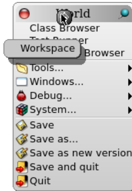
Figure 11.1: Detaching a morph, here the Workspace menu item, to make it an independent button.
