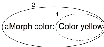
Figure 4.2: aMorph color: Color yellow is composed of two message sends: Color yellow and aMorph color: Color yellow.
